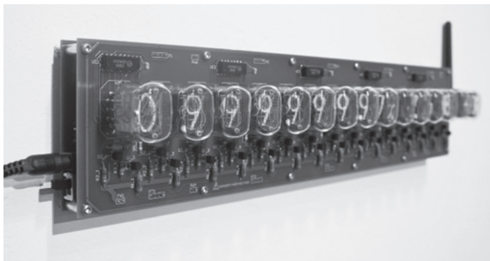
David Adey, "Omega Man (Trillion-Second-Countdown) no. 2, Countdown began: 7/1/12," 2012, Russian surplus nixie tubes, gps receiver, custom electronics, 12 identical and synchronized, 3 1/2 x 15 3/4 x 2 1/2".
